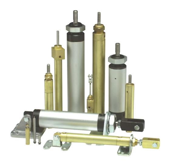
Clippard offers more types of miniature pneumatic cylinders for the designer's convenience, including: spring return, spring extend, air retract, double-acting and double rod models. From sub-miniature (5/32" bore) to heavy duty (1 1/8" bore), the extensive Clippard line provides a wide selection of bore sizes to suit any application requirement. An even wider range of strokes are available in the complete Clippard line of miniature cylinders, in stroke sizes ranging from 1/4" to 20".
